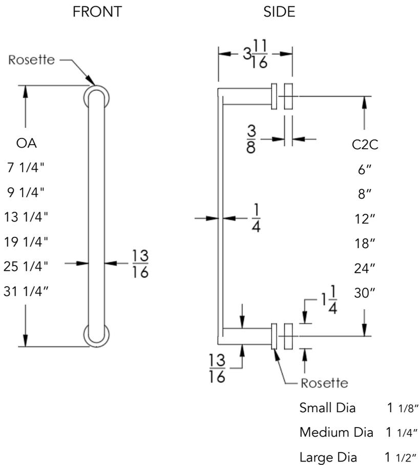
**Installation Notes:** Center to center hole drilling dimension are same as mentioned in column. Diameter of glass hole for installation is 1/2".
